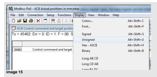
In the window the position is shown in "mm". If needed a description of the register-address can be added. For this, double-click on table cell "Alias" and enter a labelling. For this see image 16.
