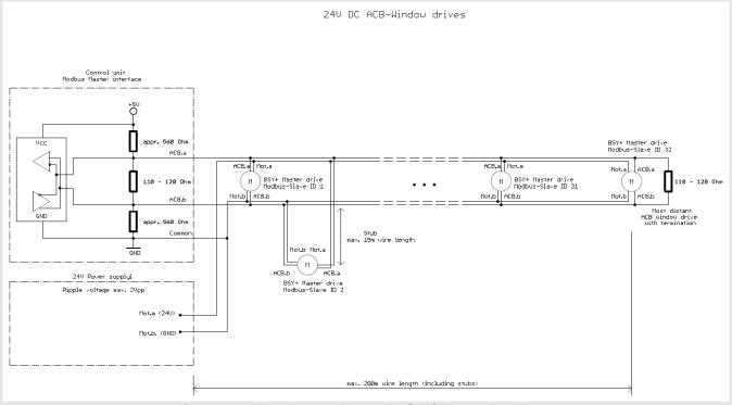
image 1 wiring diagram for 24 V DC ACB opening drives
