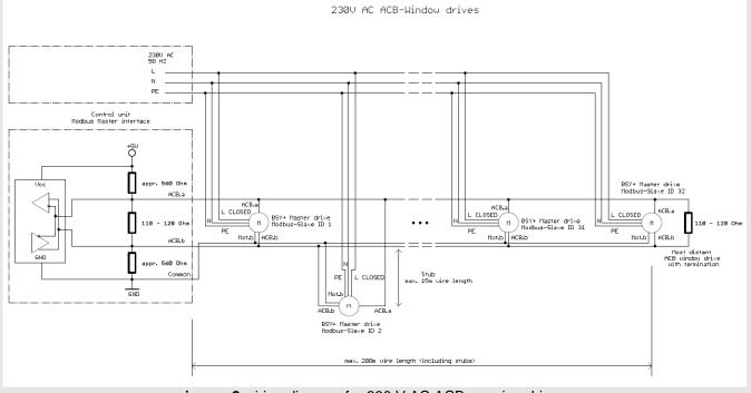
image 2 wiring diagram for 230 V AC ACB opening drives
